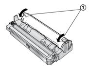
6 Make sure that the triangles (①) match, to install the toner cartridge correctly.
